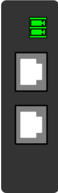
Figure. 8.9. - 41. Double RJ45 10/100 Mbps Ethernet communication module (optional). Two pin connector is IRIG-B input.
