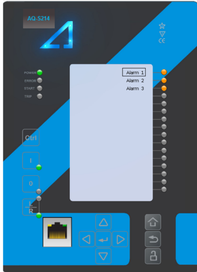
Figure. 5.2. - 29. Example situation of an alarm text and LED activation/clearing.
