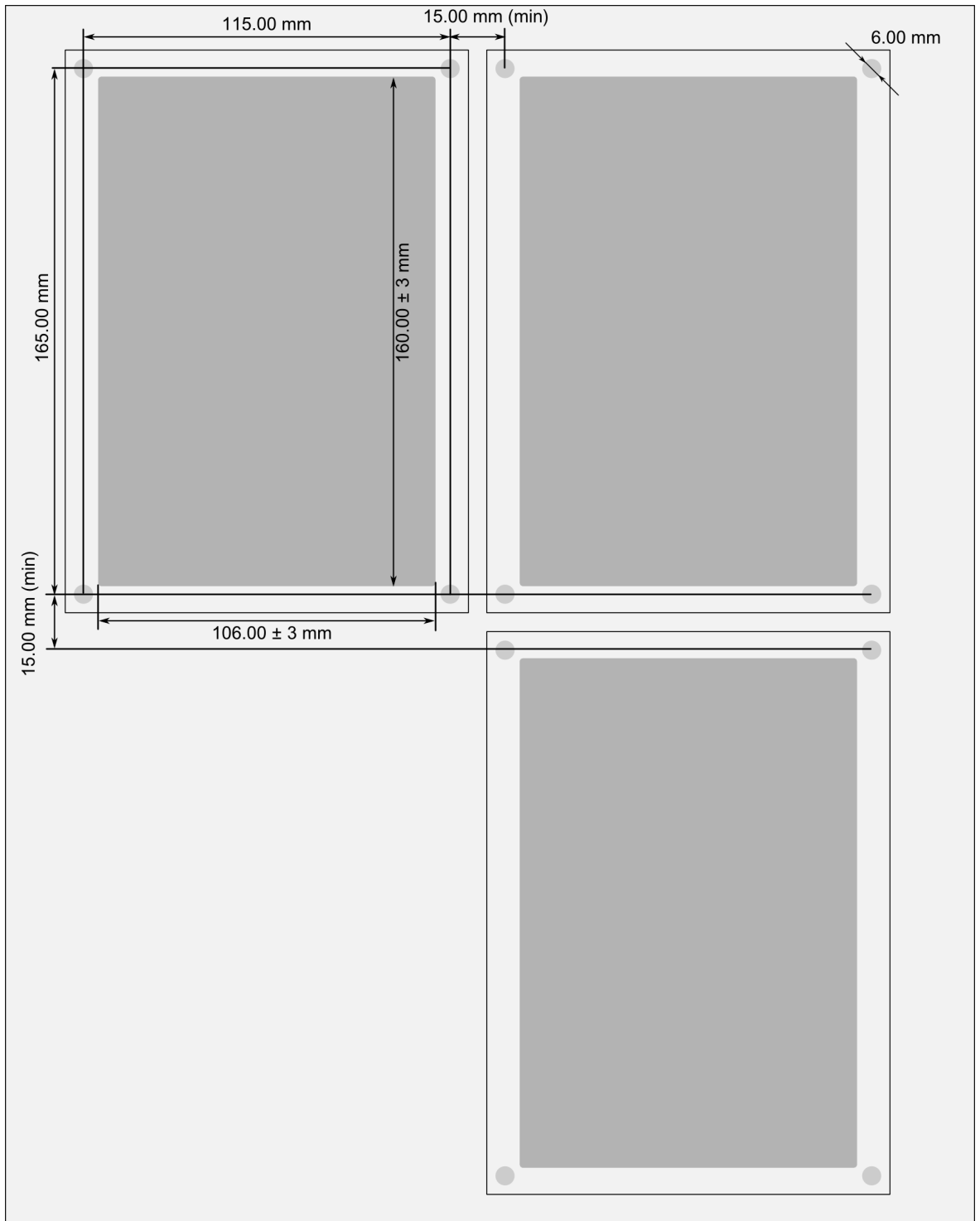
Figure. 8.10. - 67. Panel cutout dimensions and device spacing.
