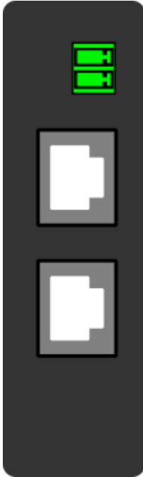
Figure. 8.9. - 62. Double RJ45 10/100 Mbps Ethernet communication module (optional). Two pin connector is IRIG-B input.
