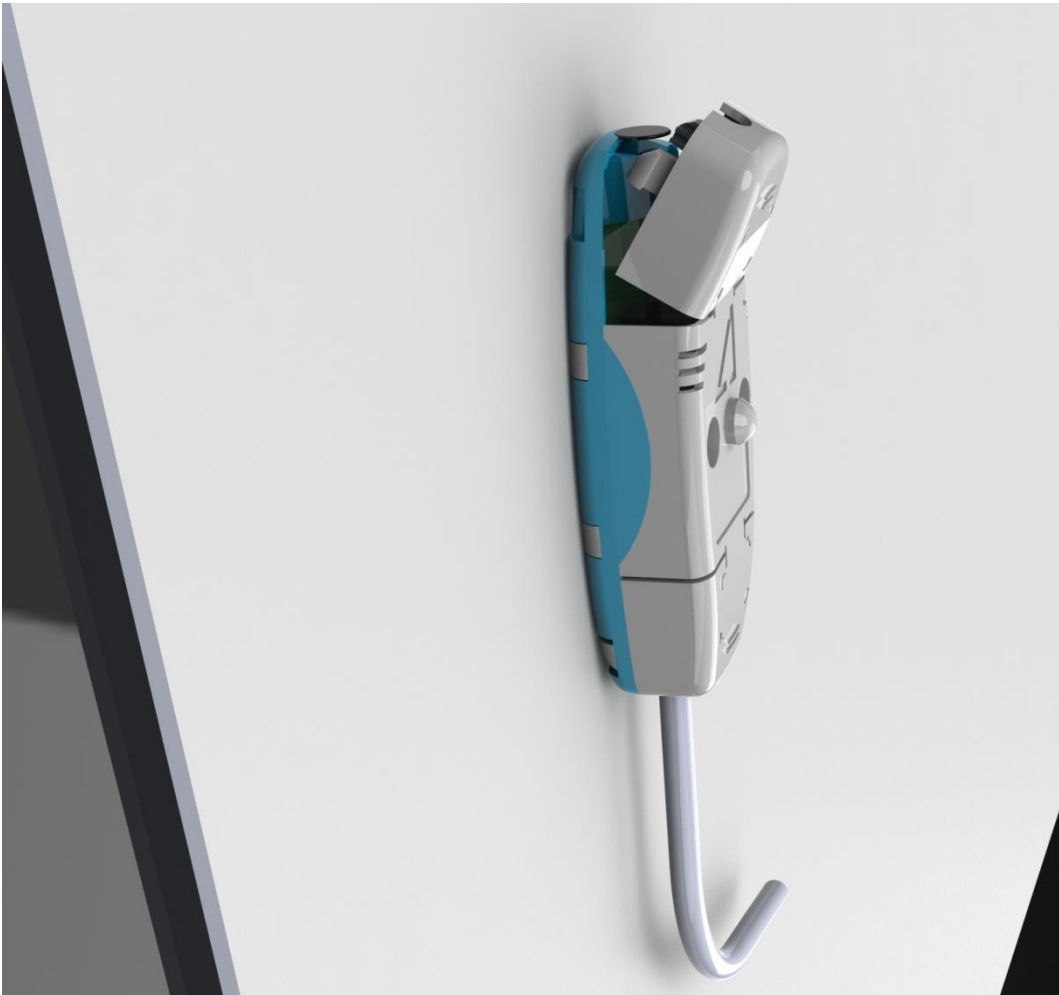
Figure 4-2: AQ 01 mounted to compartment wall.
